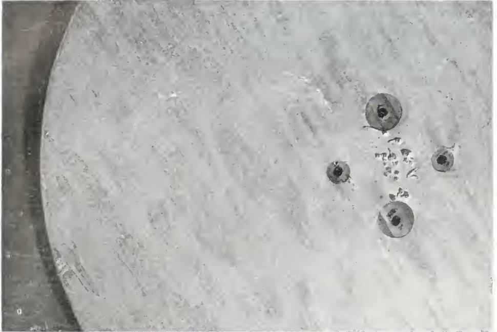
FIGURE 2. Portion of disc rotated at 192 r.p.m. for a period of 16 days, showing barnacles attached at center. Diameter of disc, 24 inches.
